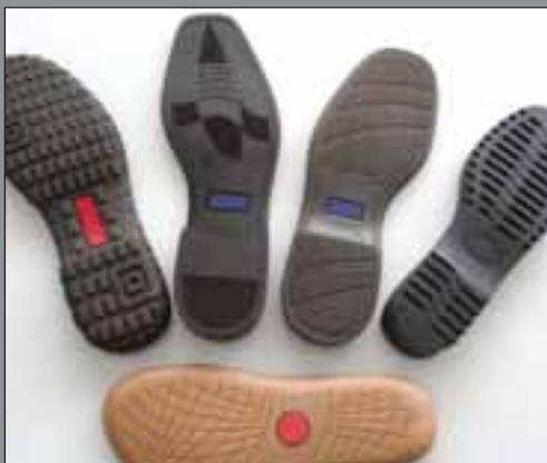
Manufacture of soles for footwear made of RUBBER, TR, PVC and TPU footwear.
